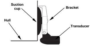
Portable transducer installed on boat transom.
